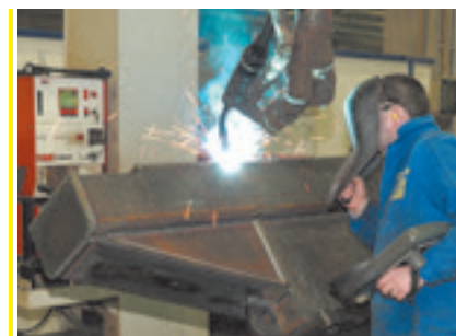
robot welding station
